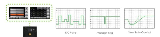
The built-in programming function of the ADG<sup>+</sup> series is consisted of GROUPs and STEPs. Users can set output voltage, output current and time to generate step or consecutive voltage/current changes, and set different rise/fall time according to their requirement. This built-in function and the ADG<sup>+</sup> series control software allow users to create complex DC waveform with sophisticated coding. Making programming the DC power supply an easy task.
