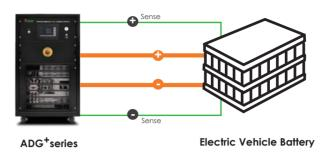
In the factory or laboratory, there is often a certain distance in the configuration of power and load. The Remote Sensing of ADG<sup>+</sup> series is able to compensate the voltage drop caused by the cable length, so the user can avoid the inconvenience of adjusting the voltage.
