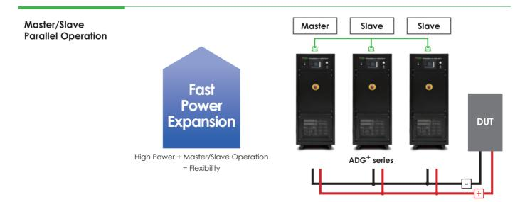
The output power of the ADG<sup>+</sup> series is up to 300kW per unit, which can be expanded to 1800kW through simple master-slave operation (max. 5 units). User can simply operate the master unit, the slave unit will receive and reply the data accordingly and equally share the load current. ADG<sup>+</sup> series is one of the few high-power DC power supply with parallel feature on the market. The availability for single-unit and parallel operation provides greater flexibility for application.
